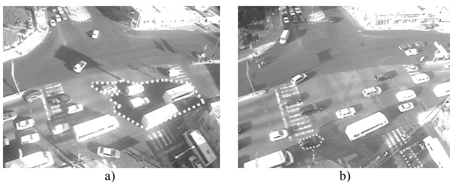
Fig. 3. Problems generated in day-time images with shadows. a) Some vehicles are merged; b) Shadows change the color of the vehicles.
