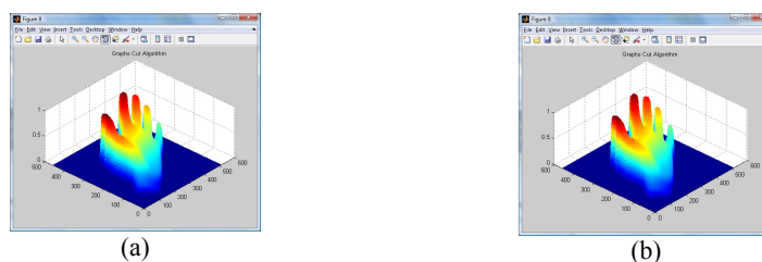
Figure 8. Reconstructed object using Morlet Wavelet and (a) Local Phase Unwrapping Algorithm, and (b) Global Phase Unwrapping Algorithm.
